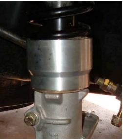
This shows the coil spacer in place notice the steel washer under the spacer. This should be installed to support the spacer.
