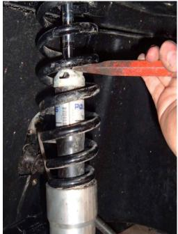
This shows how to push the strut down on the spacer. You may have to apply pressure to the strut on some installations. When you have the strut seated on the spacer tighten the lower pinch bolt.
